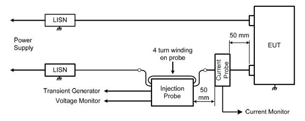
[2] Using the "Apply single Pulse" button, increase the charge voltage until either 100% of the calibration voltage is reached or the required current limit is met as measured using the current probe and current monitor.
