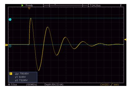
The following oscillogram shows the voltage level setting at 700V.
