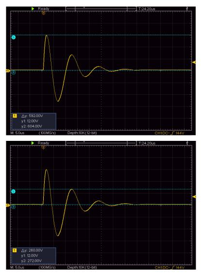
In this example, the third half cycle is 100 / 592 x 260 = 44 % which is within the required 25 % - 50 %.
